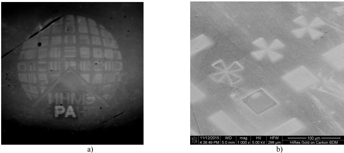
Fig.1. LSM image after developer etching (a) and SEM image of RIE silicon wafer through \text{SiO}_2 mask (b).
