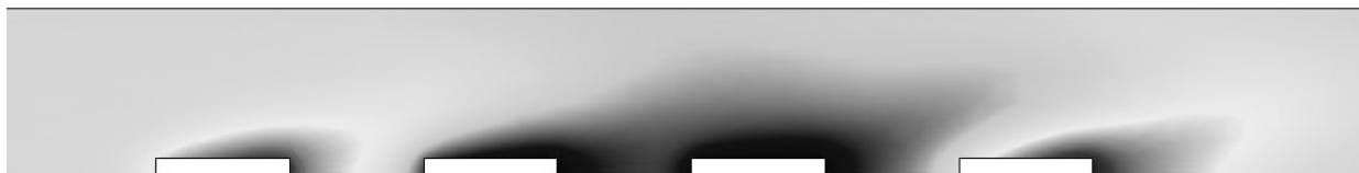
Figure 1. The calculated concentration gradient in the planar electrochemical four-electrode transducer under the condition of the high electrolyte flow.
